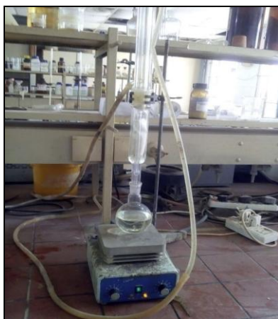
Plate 2: Experimental set up for biodiesel production by transesterification
