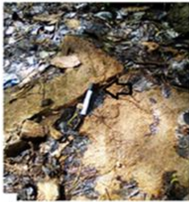
Figure 7a: Fractured Coarse grained ferruginous sandstone at Edichwa Alifokpa. Black arrow indicates the fracture
