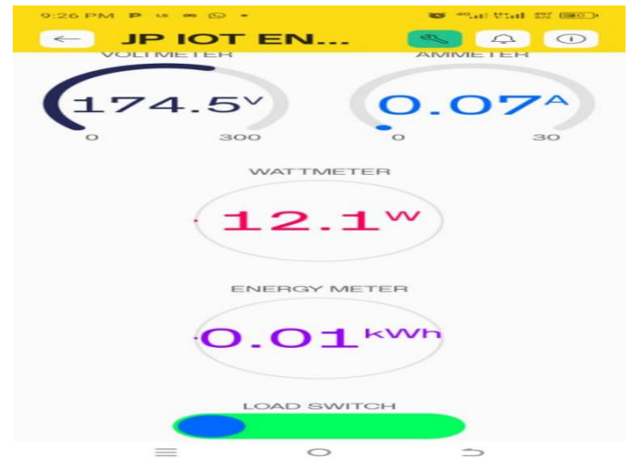
Figure 5: The energy meter cloud console on the Blynk platform showing load switch
