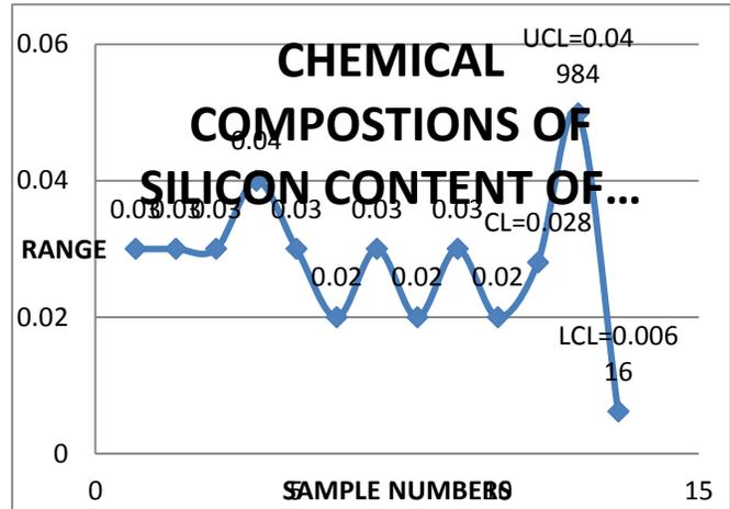
Figure 4.0 R chart: Control chart for range of chemical Compositions of Silicon content of grey cast iron
