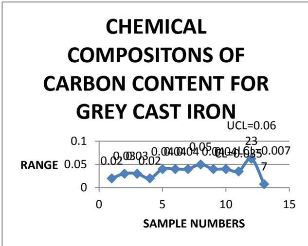
Figure 2.0 R chart: Control chart for range of chemical Compositions of Carbon content of grey cast iron.
