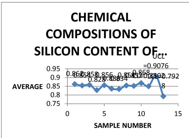
Figure 3.0 R chart: Control chart for average of chemical Compositions of Silicon content of grey cast iron
