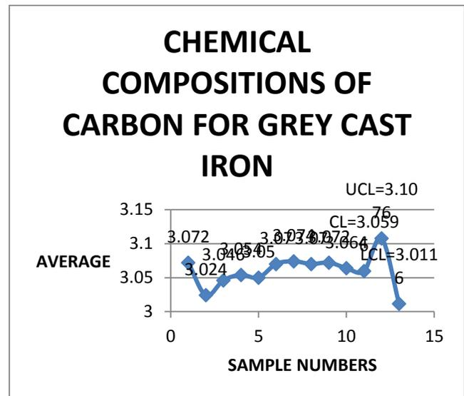
Figure 1.0 X chart: Control chart for average of chemical Compositions of Carbon content of grey cast
