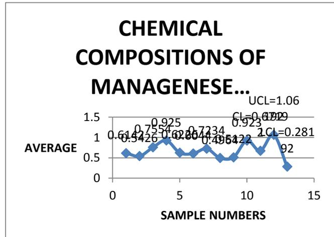
Figure 5.0 X chart: Control chart for average of chemical Compositions of manganese content of grey cast iron.
