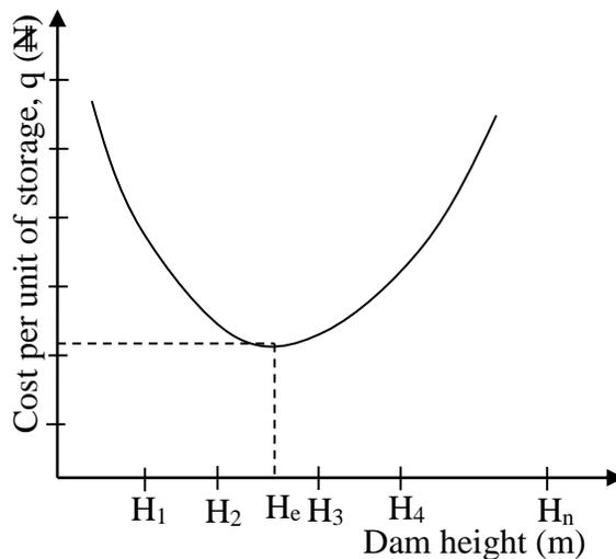
**Fig 3. Graph of cost per unit of storage versus dam height.**
