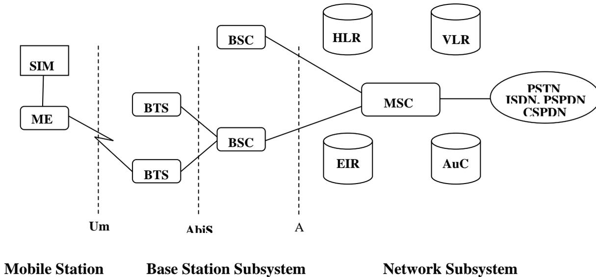
Figure 1: General Architecture of GSM Network
