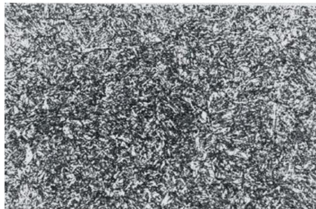
Figure 5: Microstructure of WM from SMAW.
