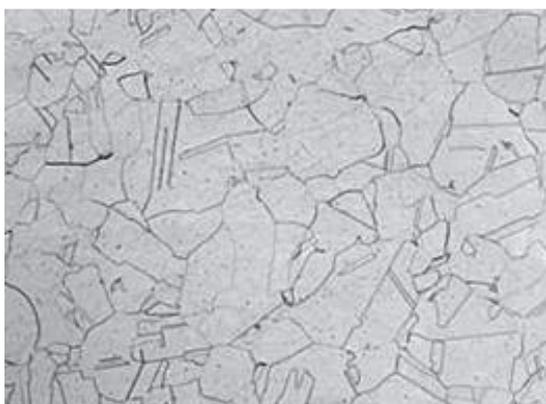
Figure 4: Microstructure of base metal (BM) before the weld -mainly austenite with retained ferrite.
