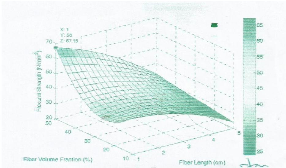
Figure 2: Flexural strength Vs fiber length and volume fraction
