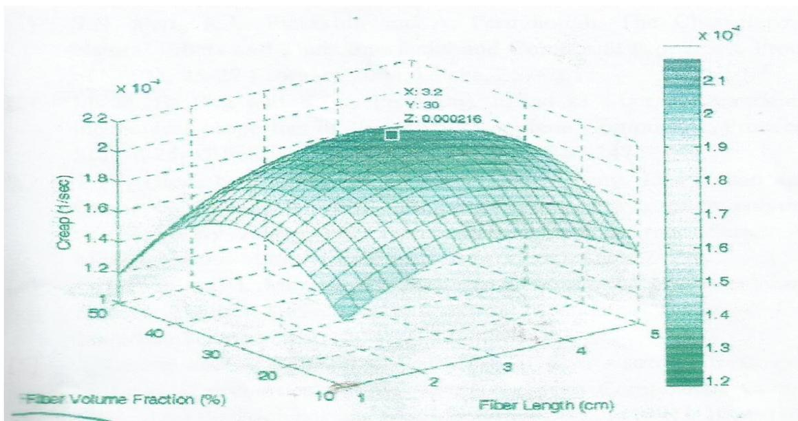
Figure 3: Creep strength Vs fiber length and fiber fraction.
