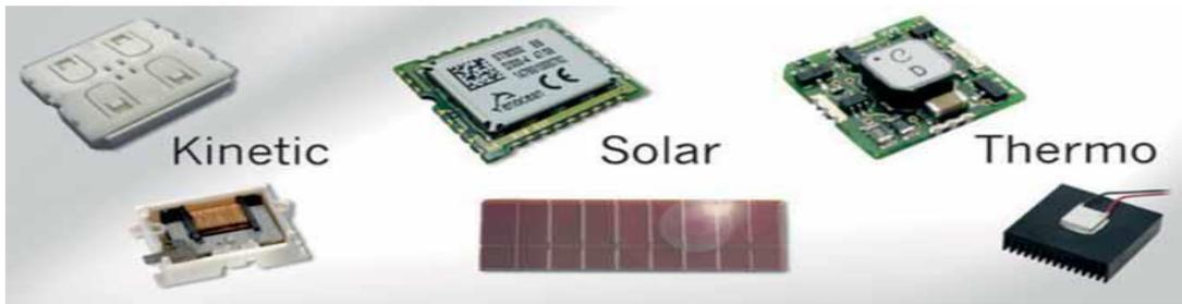
Figure 3: Sensor Nodes Configured with Ambient Energy Harvesting Devices [1].
