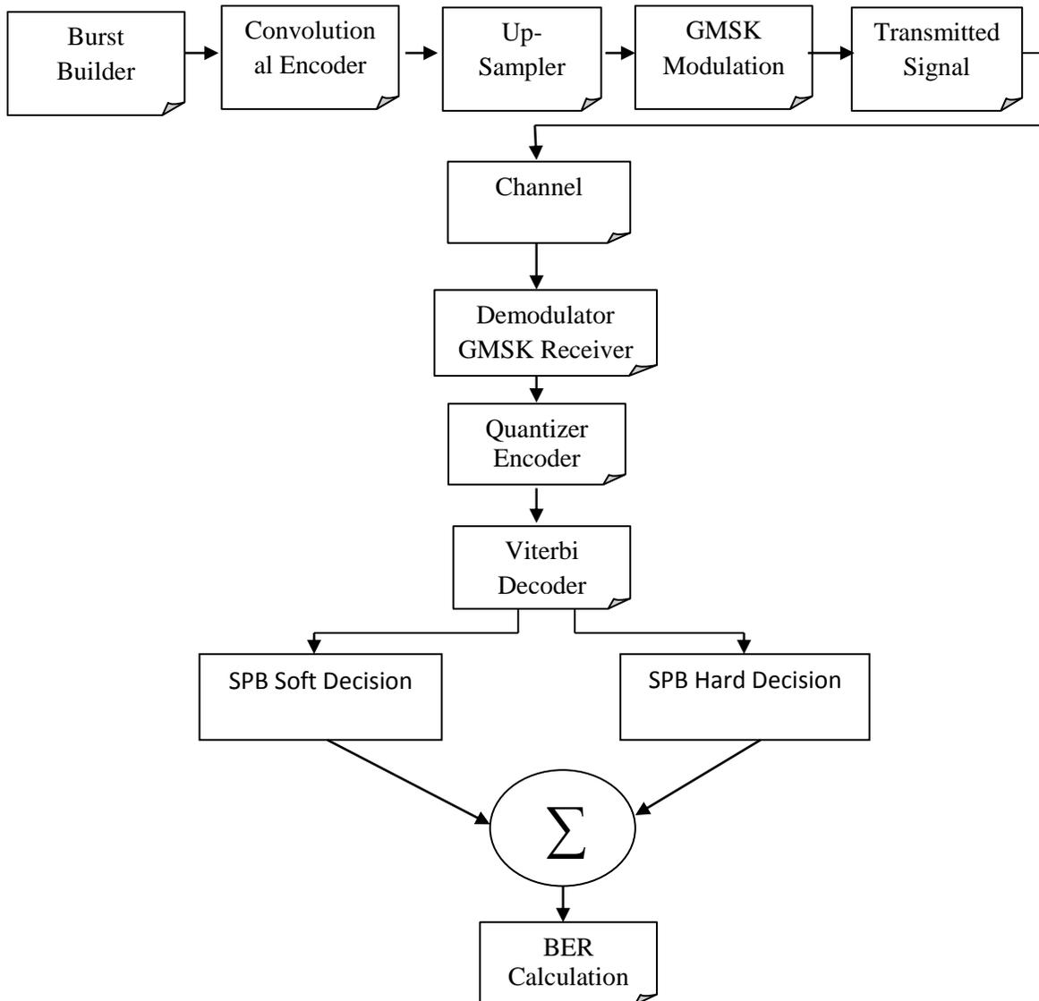
Figure 1: System Flow diagram [2]
