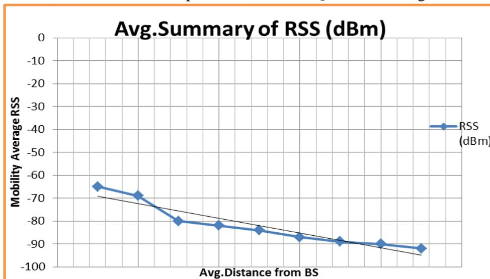
Figure 2: A Plot of Summarized Avg.RSS with Distance
