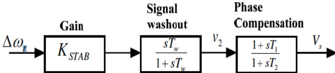
Figure 2: Block Diagram of PSS
