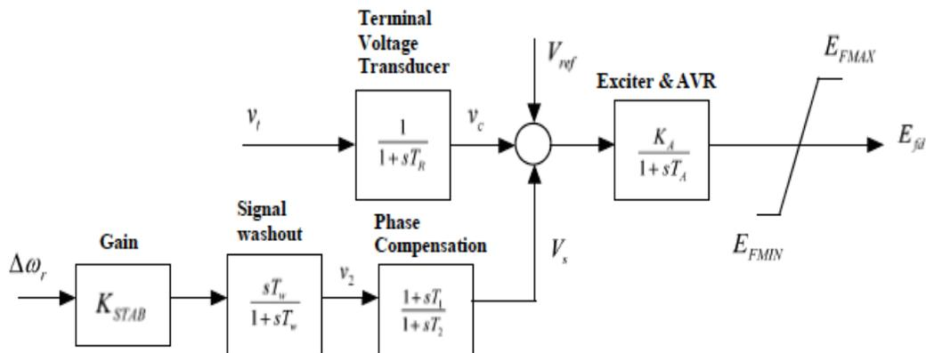
Figure 1: Block diagram of Thyristor Excitation System with AVR and PSS.
