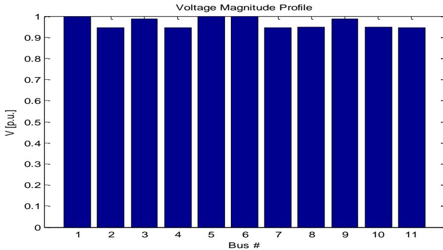
Figure 8: Voltage profile of Owerri network with PSS
