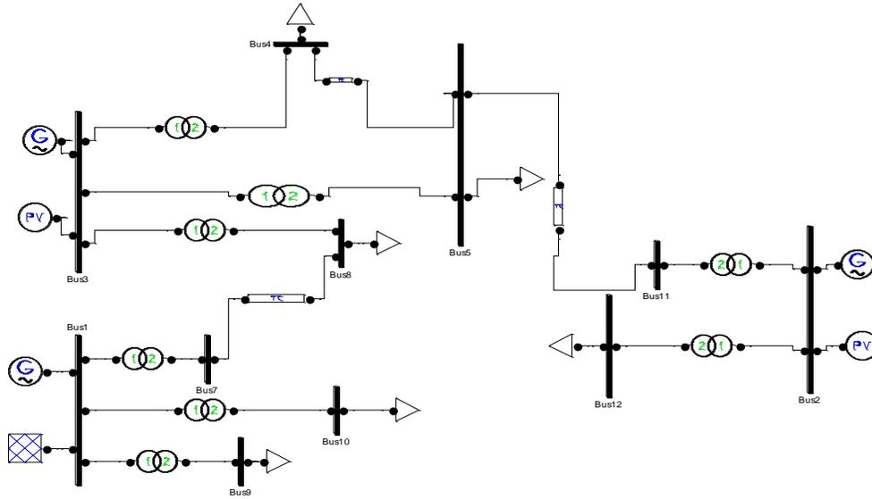
Figure 4: MATLAB SIMULINK Describing Owerri Network without PSS
