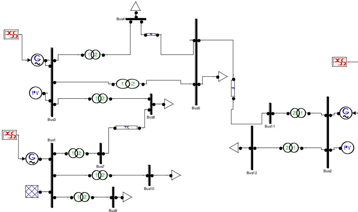
Figure 5: MATLAB SIMULINK Describing Owerri Network with PSS
