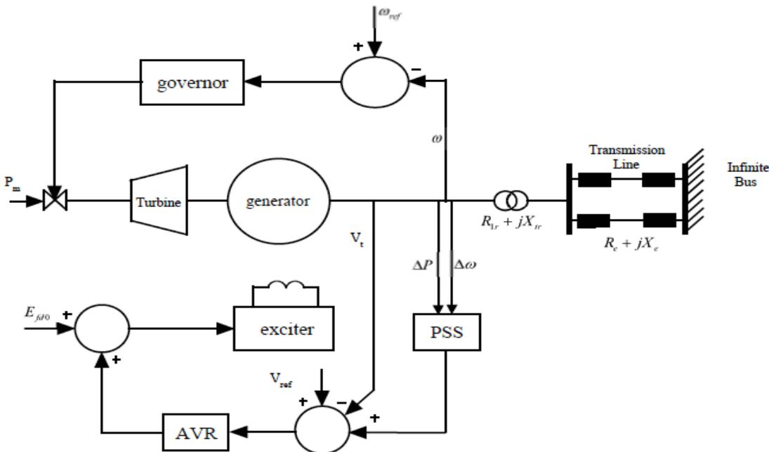
Figure 3: Power System Configuration with PSS.
