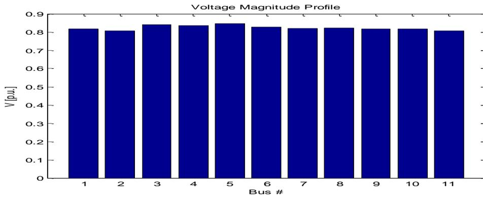
Figure 6: Voltage Profile of Owerri Network without PSS
