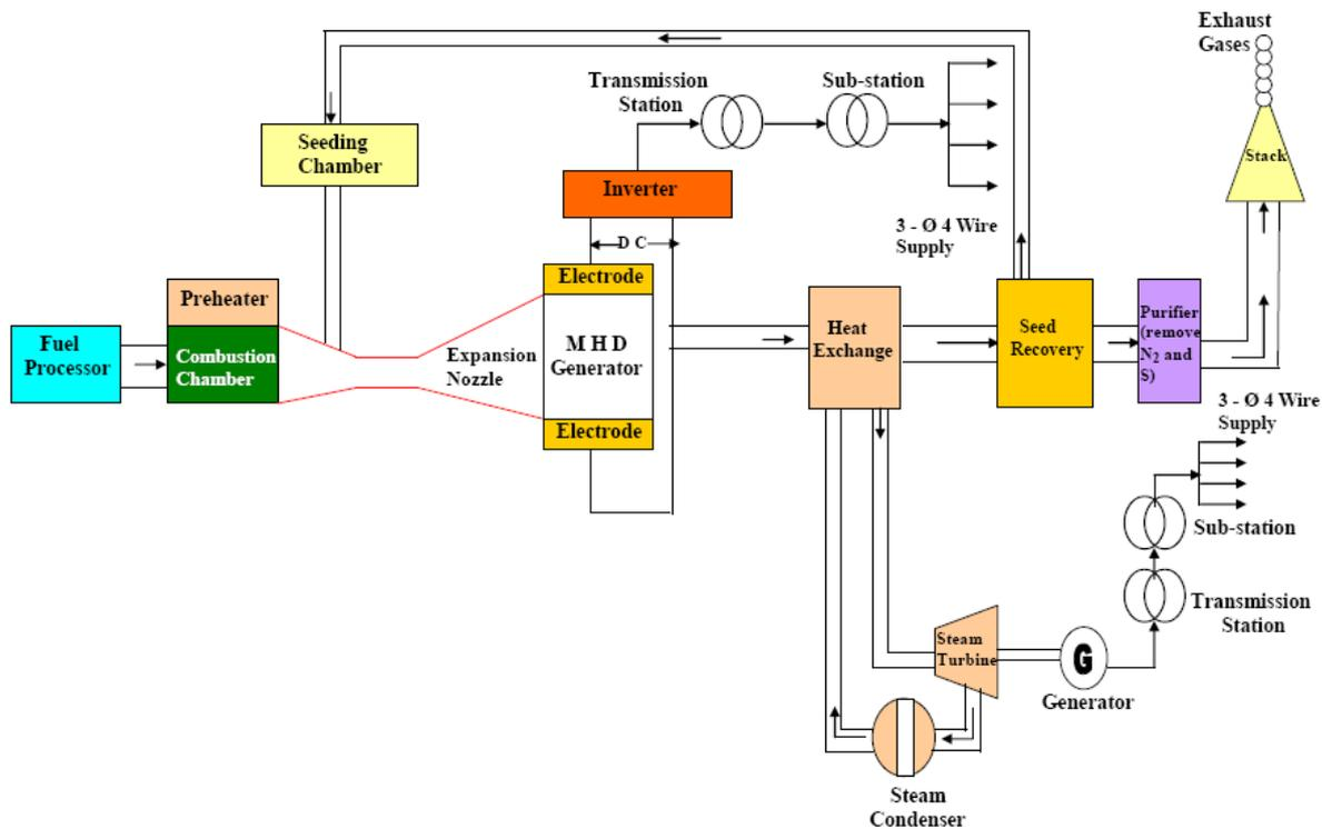
Figure 3: Hybrid Open Cycle MHD Generating Plant
