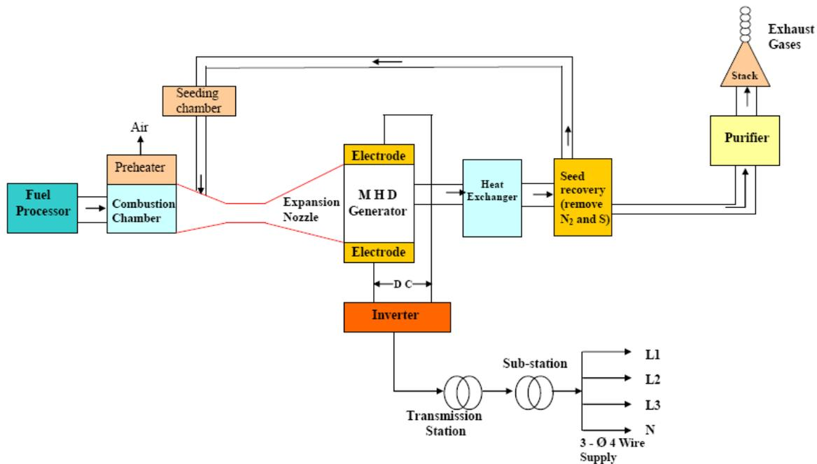
Figure 2: Open Cycle MHD Generating Plant
