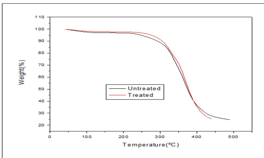
Figure 1: TGA micrograms for ramie fiber before and after alkali treatment with optimum NaOH solution
