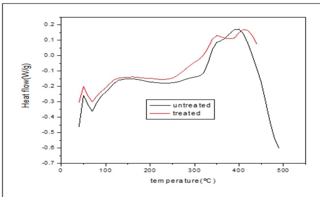
Figure 2: DSC micrograms for ramie fiber before and after alkali treatment with optimum NaOH solution
