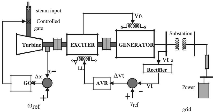
Figure 1: Control block for the power system
