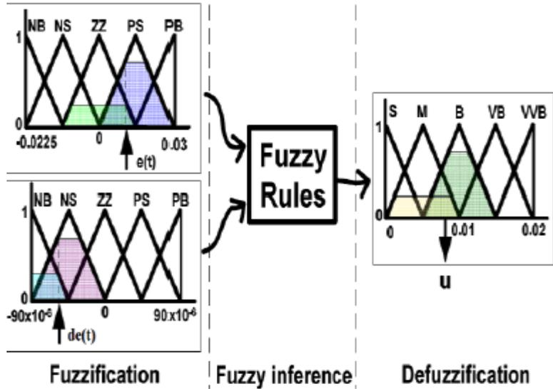
Figure 2: Fuzzy inference system for two area fuzzy controller
