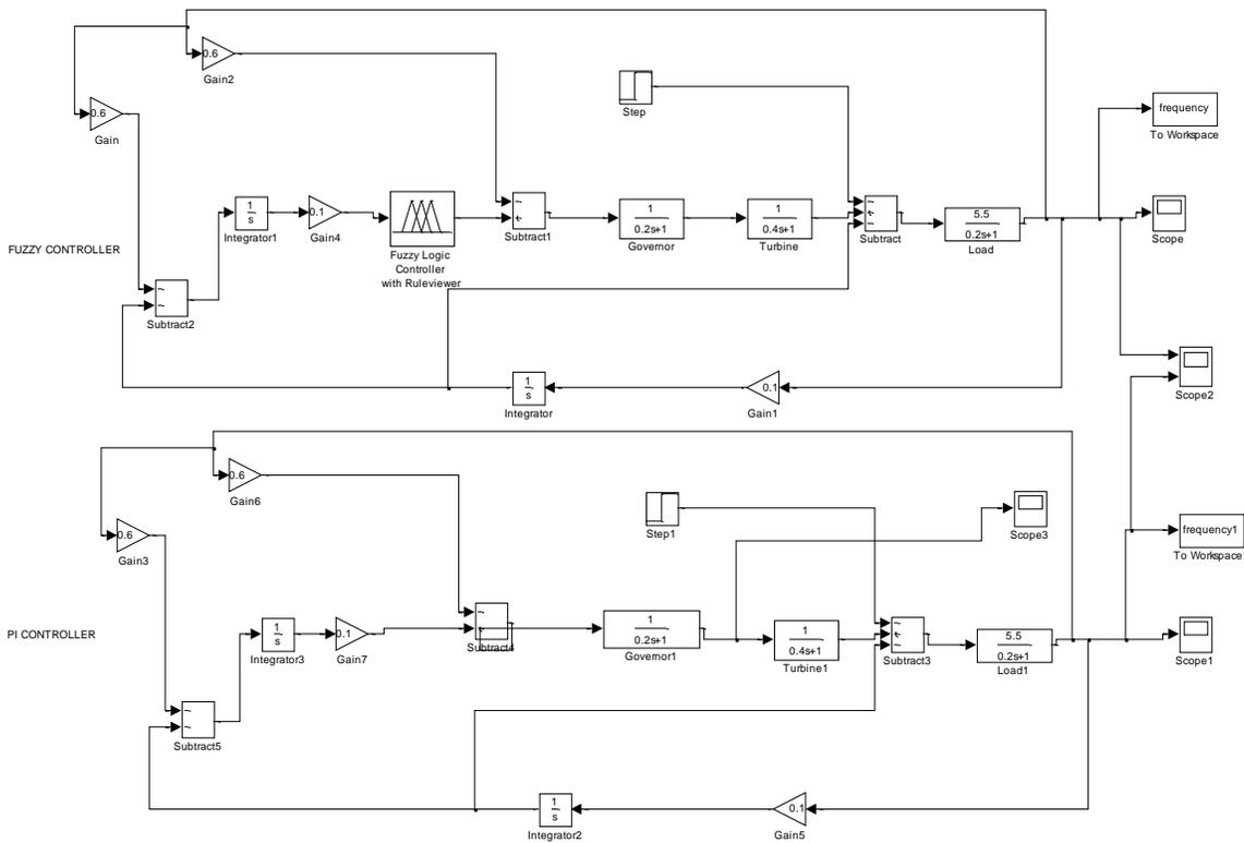
Figure 3: Simulink model for two area network using MATLAB platform
