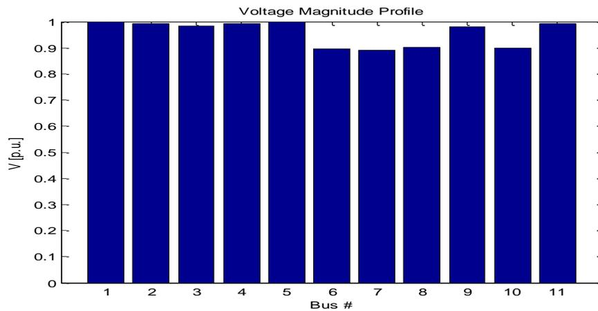
Figure 4: Voltage Profile of Imo Network Placing 25MW DG at Bus 5 (Owerri1).
