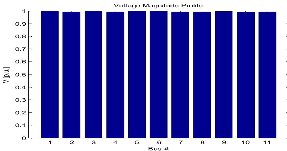
Figure 5: Voltage profile of Imo network placing 25MW DG at buses 2 (Onitsha Road) and 3 (Ahaoda).
