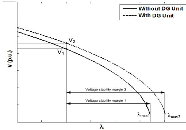
Figure 1: Impact of a DG unit on maximum Loadability and Voltage Stability Margin.
