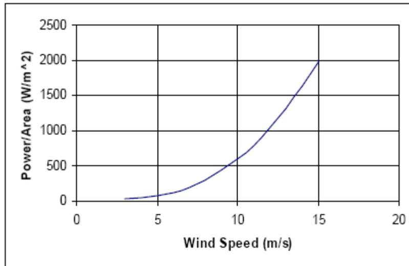
Fig. 3: Wind Power vs. Wind Speed
