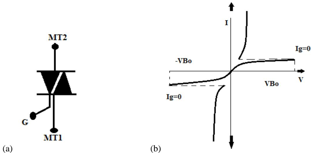
Figure 2: TRIAC symbol (a) and (b) V-I characteristic of a triac
