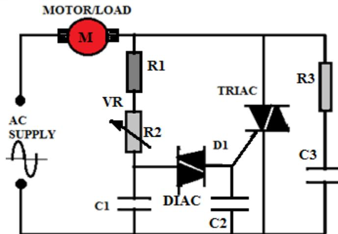
Fig. 5: Triac triggering circuit using a diac.
