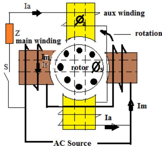
Figure 1: Single phase induction motor showing the main and auxiliary winding.
