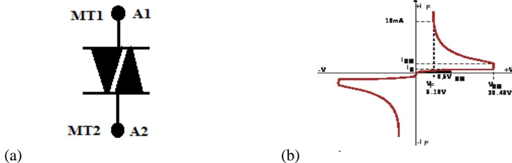
Fig 3: (a) Symbol and (b) Characteristics of DIAC
