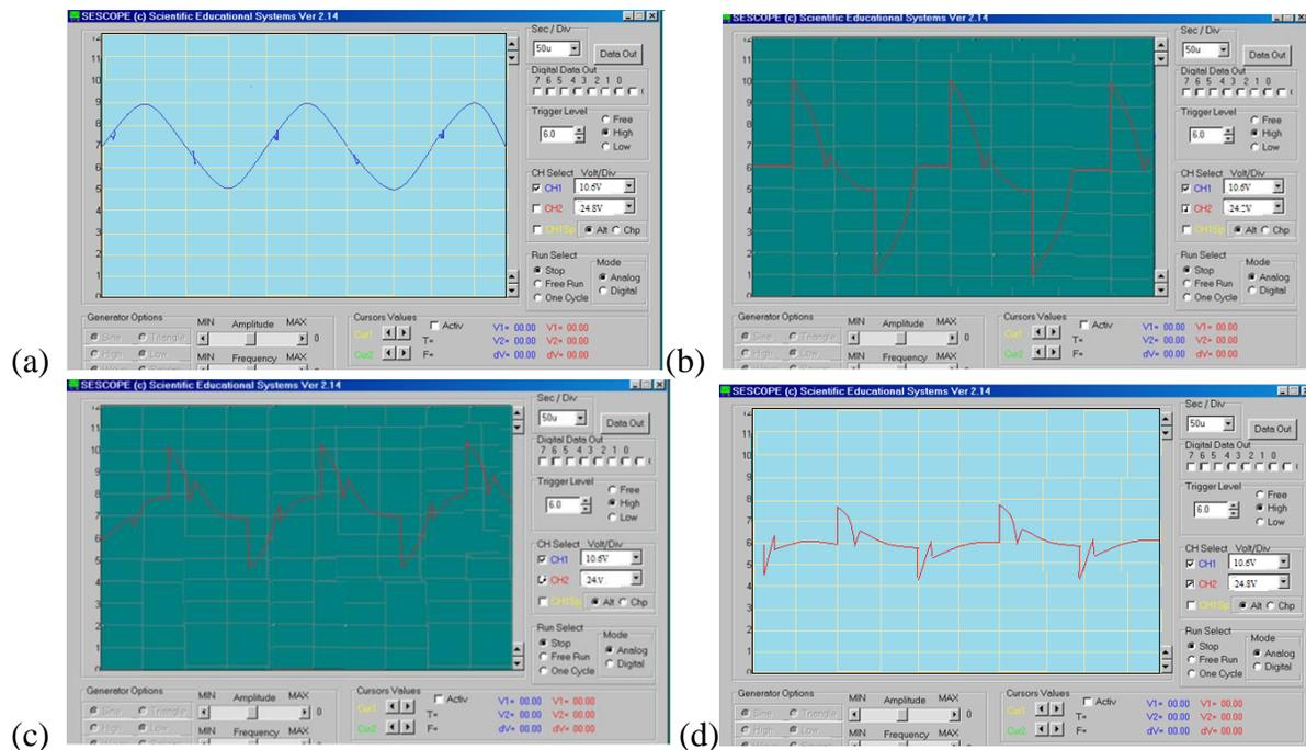
Figure 6: (a) plot between Voltage and Time at angle  $\alpha$  32.3°; (b)  $\alpha$  = 127.30°; (c)  $\alpha$  =182.4°; (d)  $\alpha$  = 212.9°
