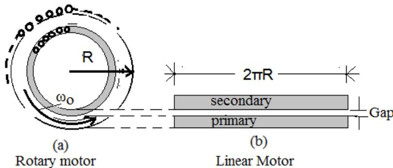
Figure 2: Radius of a rotary induction motor and length of a SLIM [Sarveswara (2015)]
