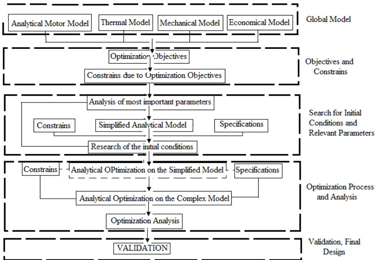
Figure 3: Schematic of an optimization process (Samuel, 2016).
