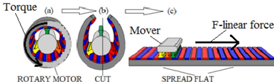
Figure 1: Imaginary process of unrolling a conventional motor to obtain a LIM
