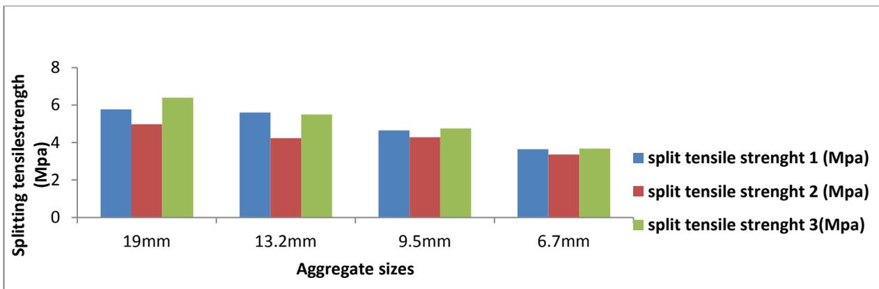
Figure 4.4: 28 days Splitting Tensile Strength Result
