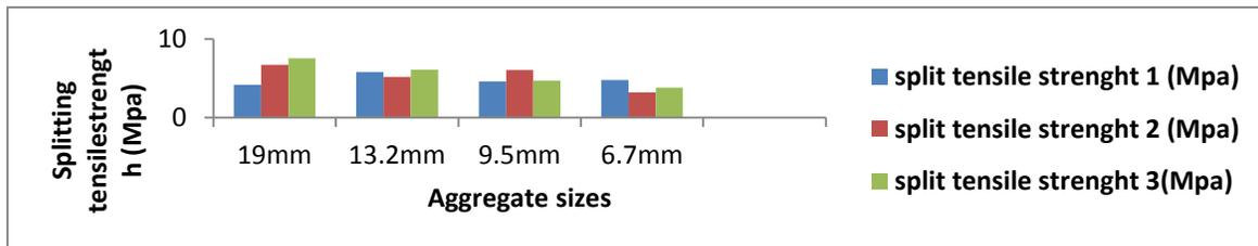
**Figure 4.2: 14 days Splitting Tensile Strength Result**
