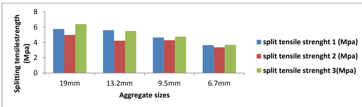
**Figure 4.1: 7 days Splitting Tensile Strength Result**
