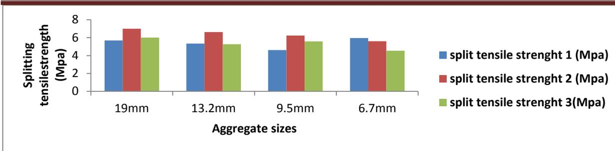
Figure 4.3: 21 days Splitting Tensile Strength Result
