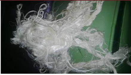
Fig.3 Extracted sisal fibre
