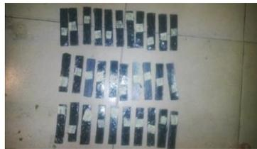
Figure 6: Flexural test samples
