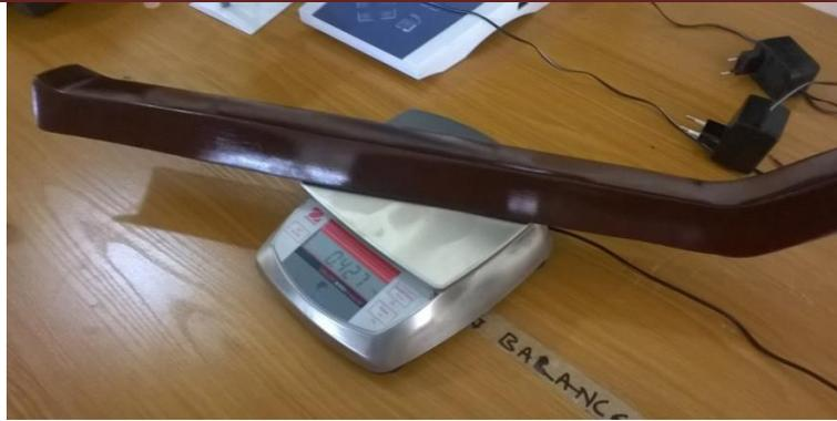
Figure 14: Finished Chassis panel weighs 421grams
