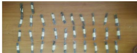
Figure 8: Impact test samples
