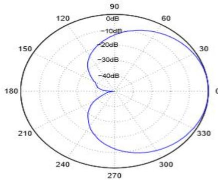
Figure 1: Switched Beam Pattern
