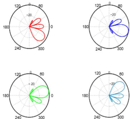
Figure 3: Resultant radiation pattern of practical array of 4 elements (clock wise from top left for  $\theta_s = -45^0, -15^0, 15^0$ , and  $45^0$ ).
