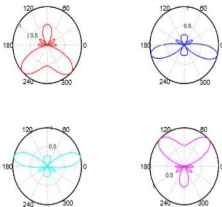
Figure 2: Array factor (clock wise from top left for  $\theta_s= -45^0, -15^0, 15^0$  and  $45^0$ )
