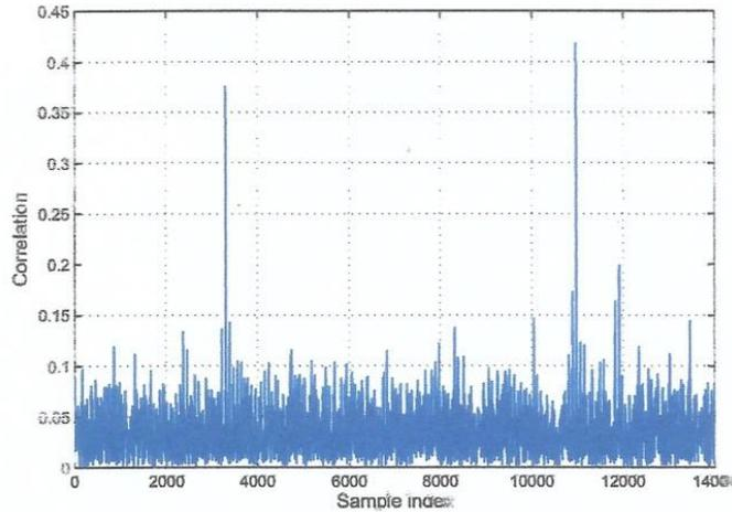
Figure 3: XCF for TTI of 2 Slots in UFMC with SNR of 0dB.
