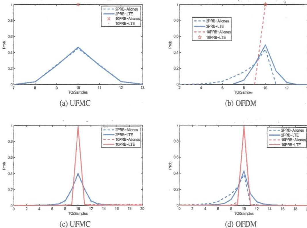
Figure 4: UFMC and OFDM Timing Offset Estimator Performance.
