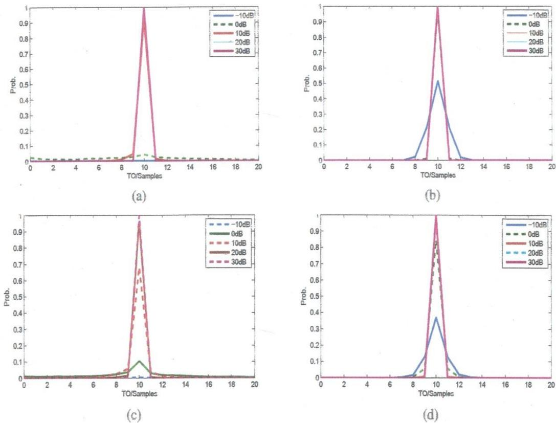
Figure 5: CP-based and Pilot-based Timing Estimator in OFDM
