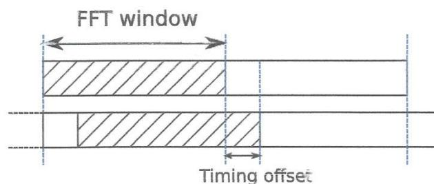
Figure 1: Timing Offset between Transmitter and Receiver
