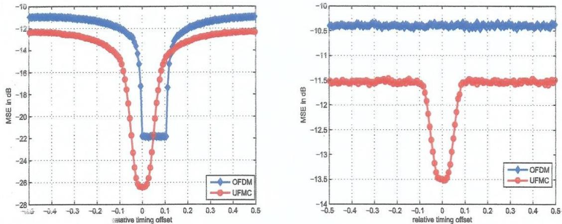
(a) Effect of timing offset in UFMC and OFDM under rCFO 0.1 subcarrier spacing
