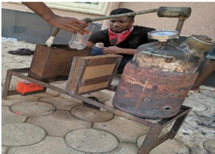
Plate 1: The Pyrolysis set-up employed for the thermal degradation of waste polymers.
