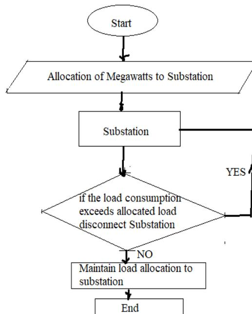
Figure 1: Flow chart of the model for automatic network control technique
