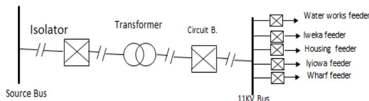
Figure 2: Single line of a distribution network architecture
