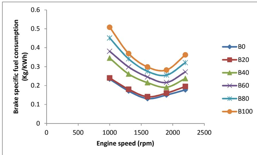
Figure 2: Effect of engine load on brake specific consumption for diesel, RSOFAME and blends
