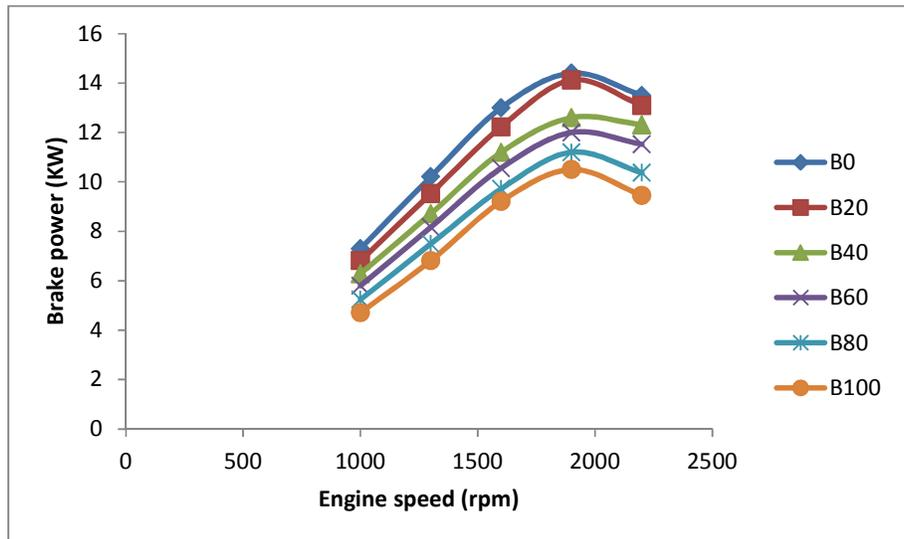
Figure 4: Effect of engine speed on brake power for diesel, RSOFAME and blends
