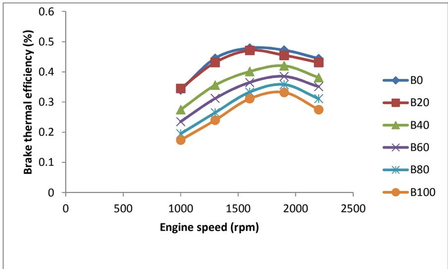
Figure 3: Effect of engine speed on brake thermal efficiency for diesel, RSOFAME and blends
