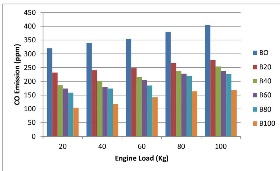
Figure 6: Effect of engine load on CO emission for diesel, RSOFAME and blends
