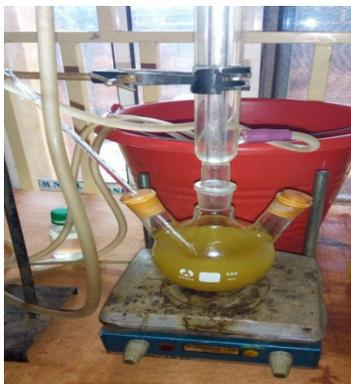
Plate 1: Biodiesel production by transesterification of oil
