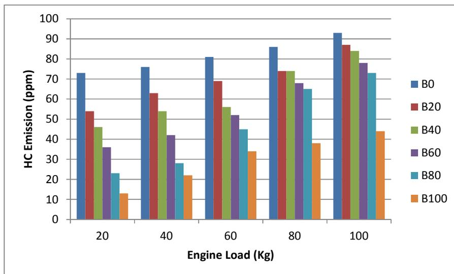
Figure 7: Effect of engine load on HC emission for diesel, RSOFAME and blends
