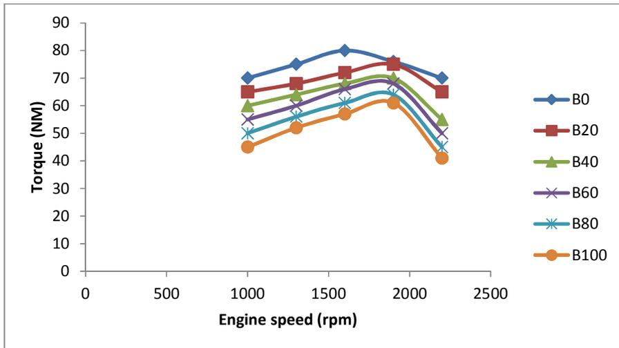
Figure 1: Effect of engine speed on torque for diesel, RSOFAME and blends
