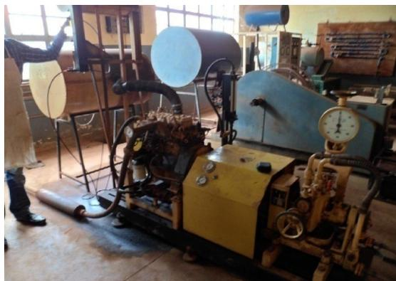
Plate 2: Perkin 4:108 diesel engine mounted on Steady state engine test bed at UNN Nsukka
