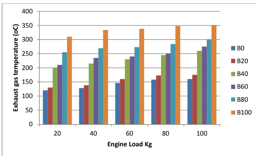
Figure 5: Effect of engine load on exhaust gas emission for diesel, RSOFAME and blends
