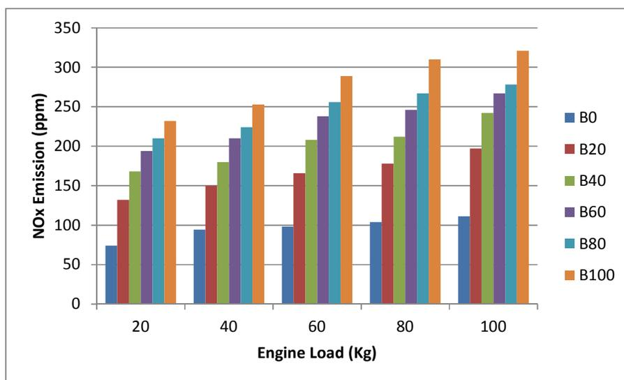
Figure 8: Effect of engine load on NOx emission for diesel, RSOFAME and blends
